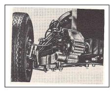
The Healey designed "trailing arm" front end suspension was developed to help his fast, low sports cars hold the road on curves and aid the driver in steering at all times. The front wheels are mounted on pivoting arms ahead of the wheel center line. This arm is cushioned against a coil spring. In taking bumps, each wheel deflects vertically in an arc without change to tread or camber
