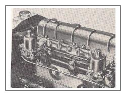
As modified by Healey, the 234.8 cid Ambassador six was rated at 125 bhp at 4000 rpm. Providing the extra horsepower was a pair of British SU sidedraft carburetors, a hotter cam and an aluminum cylinder head with sealed intake manifold and an 8.0:1 compression ratio
